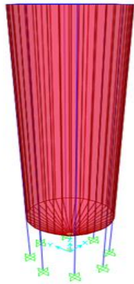
Fig.1 R.C.C. Silo without shear wall
