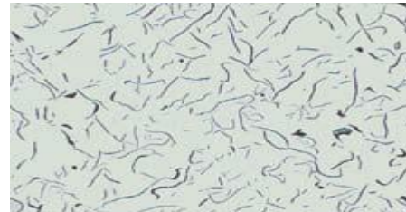
Fig. 2: showing correct polish 200x
