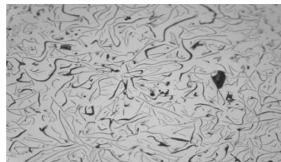
Fig.3. Microstructure of Gray iron under a 100x microscope
