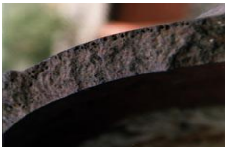
Fig 3a. Gray surface after fracture
