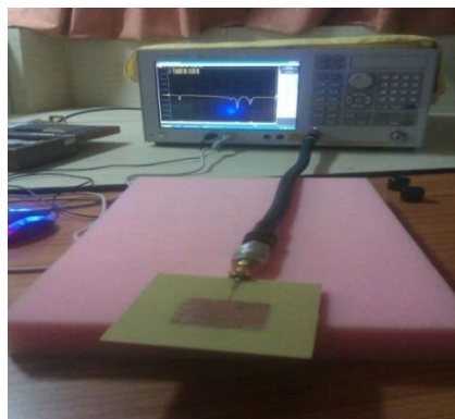
Figure 6.2.4: Fabricated antenna on 2 nd iteration
