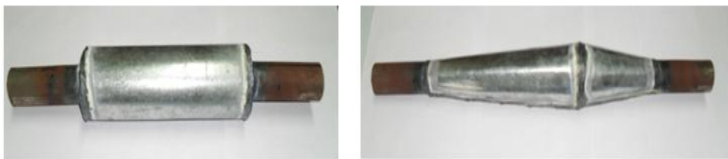
Fig 2 Actual Catalytic converters (Cylindrical & Convergent-Divergent shape)
