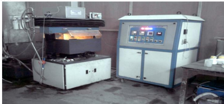
Fig 3. Experimental set up of ECM process
