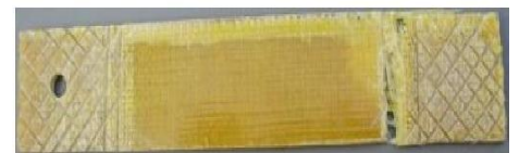
Fig. 13.1 Tensile Test Specimens of Glass Fiber Epoxy, Chapsten E-Glass Epoxy and Glass Fiber Polyester Epoxy
