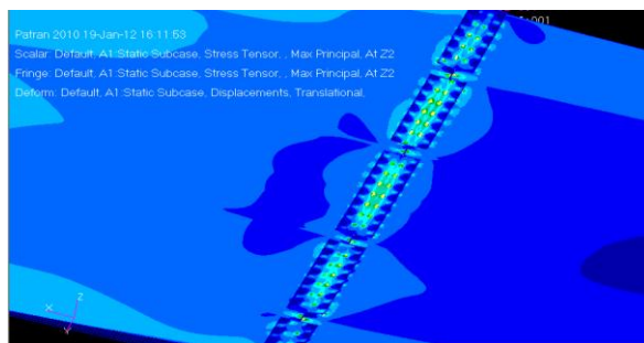
Figure 3(b) maximum stress concentration at bottom skin splice joint
