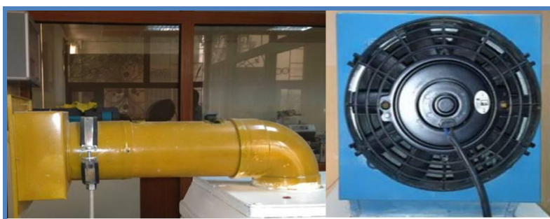
Figure (2): The air outlet duct and the used fan, the air inlet duct.
