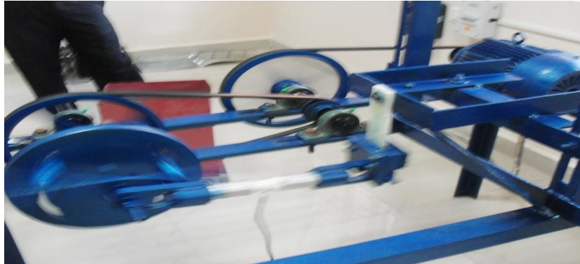
Fig 1. Positioning of composite material in vertical direction in Pictorial view of Fatigue Test Rig
