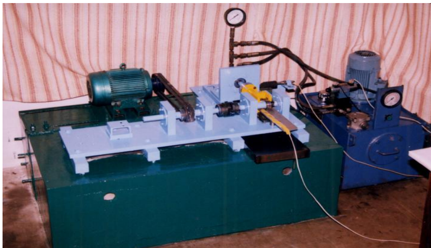
Fig 2. Positioning of composite material in horizontal direction in Pictorial view of Fatigue Test Rig
