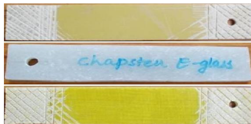
Fig. 13.1 Tensile Test Specimens of Glass Fiber Epoxy, Chapsten E-Glass Epoxy and Glass Fiber Polyester Epoxy
