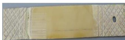
Fig. 13.2 Glass Fiber Epoxy Specimen after Tensile Test
