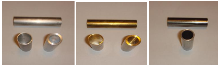
Figure 6: Initial tube shapes for the aluminium alloy, brass and steel
