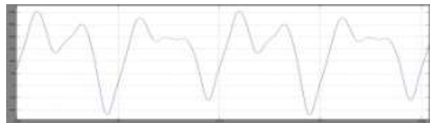
Figure 11: Speed waveform (Period Two) for 100 Volt (R.M.S)
