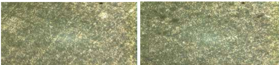
Fig.6 Microstructure variation of Eutectoid steel before and after friction welding at 675x.
