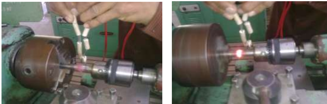
Fig. 3. The locations of the thermocouple placement 7, 14, 21 and 24mm from the interface, respectively.
