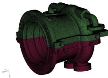
Fig 3.2: Steam Casing (HP) Meshed Model
