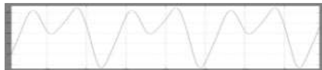
Figure 11: Speed waveform (Period Two) for 100 Volt (R.M.S)
