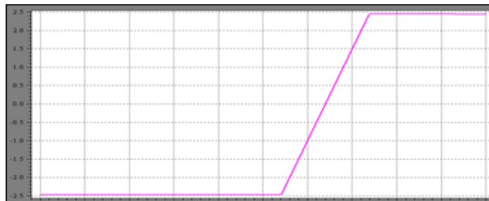
Fig.14 Transfer Function Of Linear Function With Adjustable Threshold
