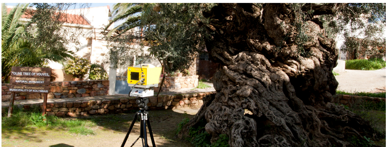
Figure 4. 3D scanning of the outer surface of the trunk
