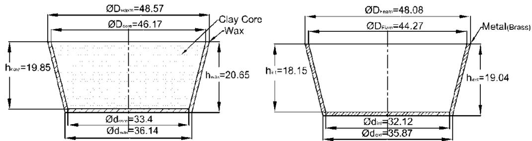
Fig. 3.11: Schematic diagram of Cosmetic Case with Dimension in different stage of production. Clay Core and Wax pattern (Top), Cast Sample (Bottom)
