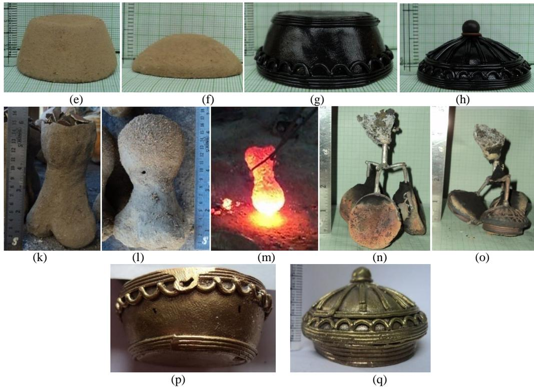
**Fig.2.1:** Steps of cosmetic case and cap casting: (a, b) Schematic diagram Cosmetic Case (Left) and its Cap (right), (c) Dies, (d) working artisan, (e, f)- core, (g, h)- Thin Walled Wax Pattern, (i) Gating on wax Pattern, (j) Primary Clay Coating, (k) clay mold with brass scrap, (l) Covered clay mold, (m) Fired mold- pouring of liquid metal also done, (l, m) Samples with Gating System, (p, q)- finished casting product.
