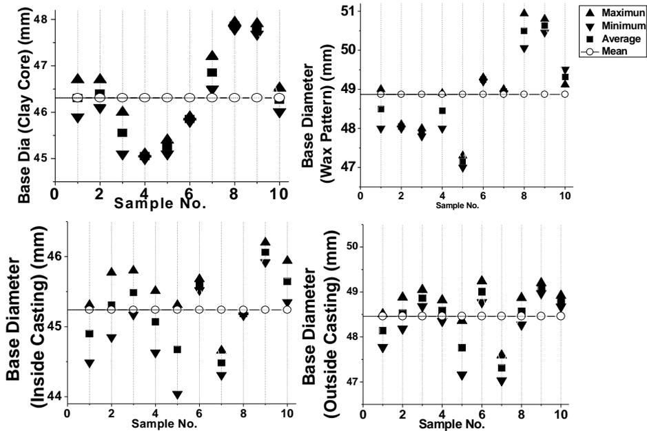
Fig.3.6: Distribution of Major, Minor, Average and mean Diameter of Base for Clay core, Wax Pattern, Inside and outside measurement of Cosmetics Cap
