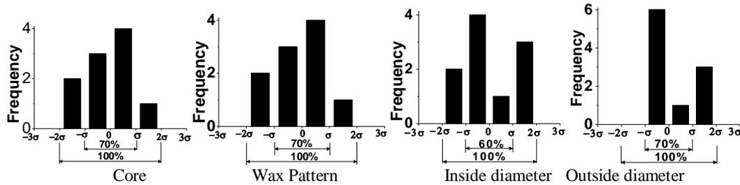
Fig.3.5. (a) Frequency Distribution of core, wax pattern, internal and external Lip Diameter
