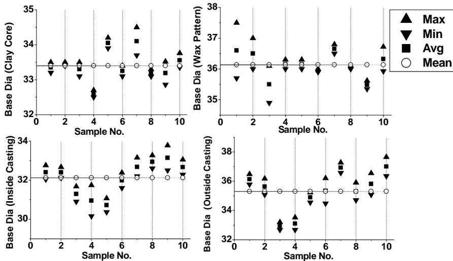
Fig.-3.2: Distribution of Major, Minor, Average and mean Diameter of Base for Clay core, Wax Pattern, Inside and outside measurement of Cast products.
