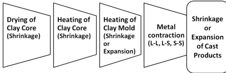
Fig.-3.10: Shrinkage/ Expansion of Mold and Metal at different stages of Production
