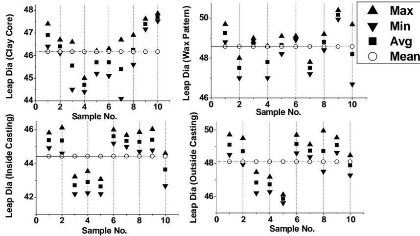
Fig.-3.1: Distribution of Major, Minor, Average and mean Diameter of Lip for Clay core, Wax Pattern, Inside and outside measurement of Cast products.
