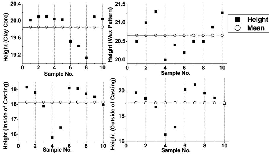
Fig.-3.3: Distribution of Height and mean height of Clay core, Wax Pattern, Inside and outside measurement of Cast product.
