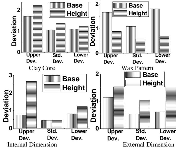
Fig.3.8: Upper, Lower and Standard deviation of (a) clay core, (b) wax pattern, (c) Internal and (d) External dimensions of container cap.
