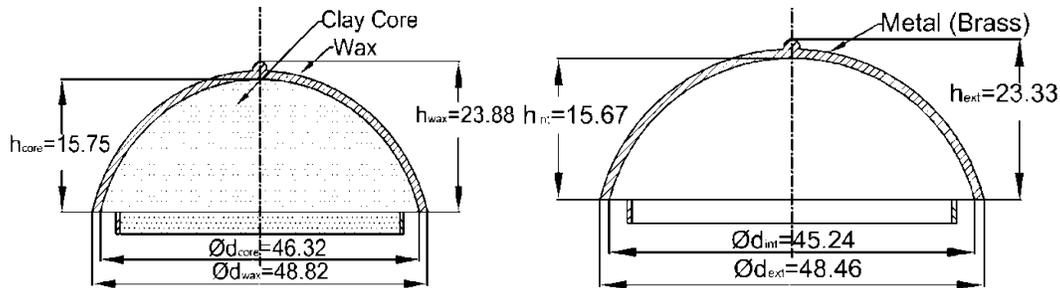
Fig. 3.12: Schematic diagram of small powder case cap in different stage of production.
