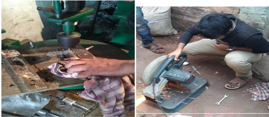
[Figure 20: Cutting & Drilling the wheel shaft]
