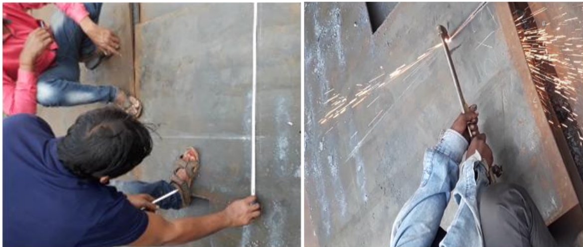
[Figure 19: Cutting of Sheet metal]
