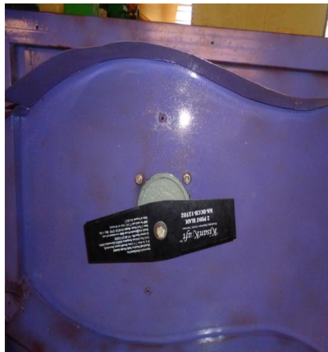
[Figure 23: Blade fixed with motor Shaft]
