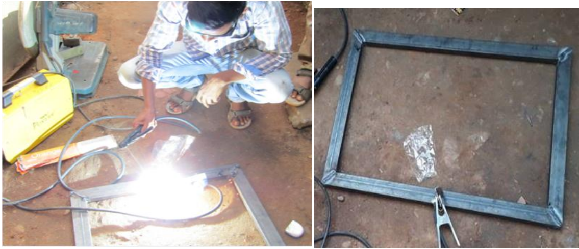
[Figure 18: welding of Base Frame]
