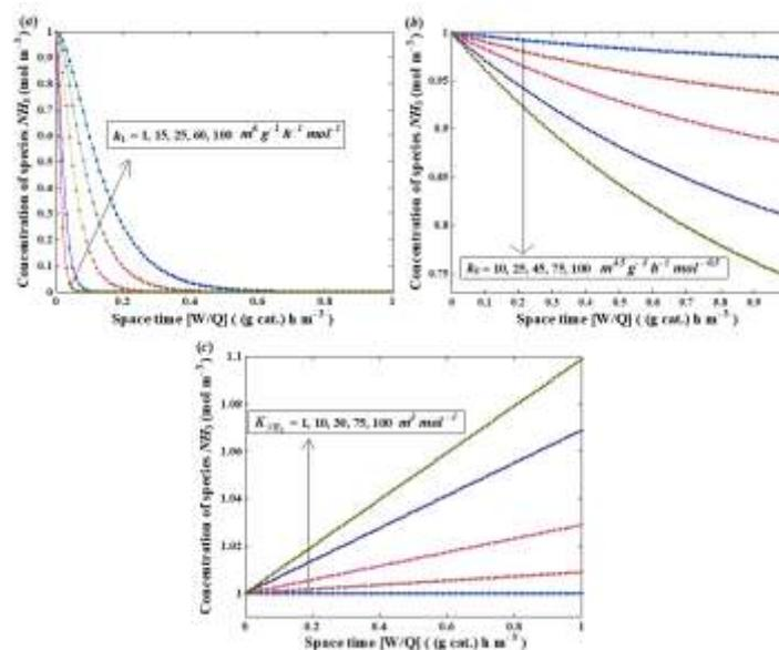
Figure.1 Plot of concentration of species NH<sub>3</sub> versus Space time [W/Q] with various values of the parameters and some fixed values all other parameters.
