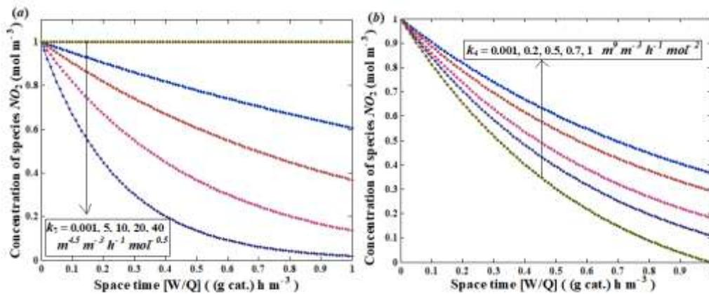
**Figure.3** Plot of concentration of species  $\text{NO}_2$  versus Space time  $[\text{W}/\text{Q}]$  for various values of the parameters and some fixed values all other parameters.
