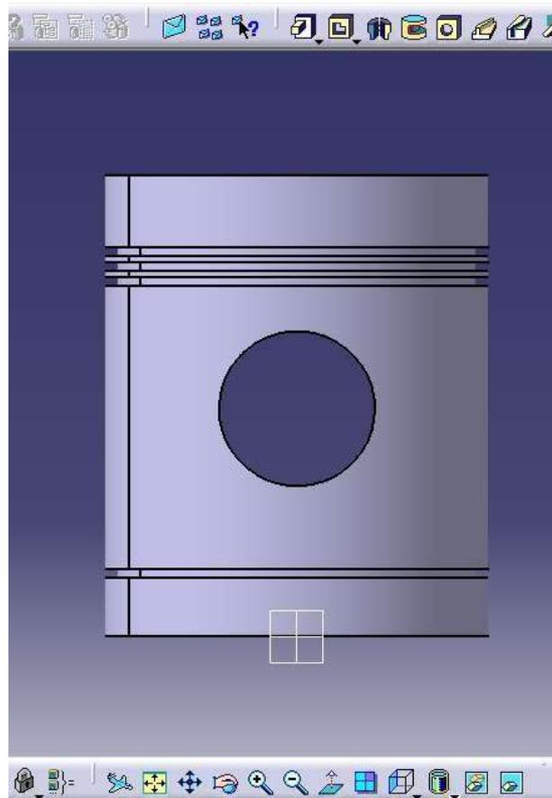
**Fig.2** Piston head modeled in CATIA V5R20 based on above calculations
