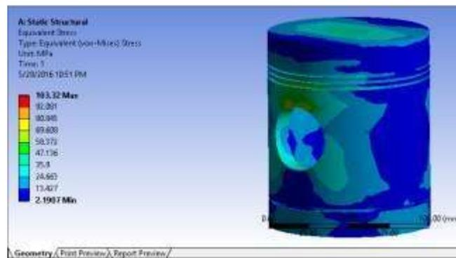
Fig.7 Results obtained for stress in piston head
