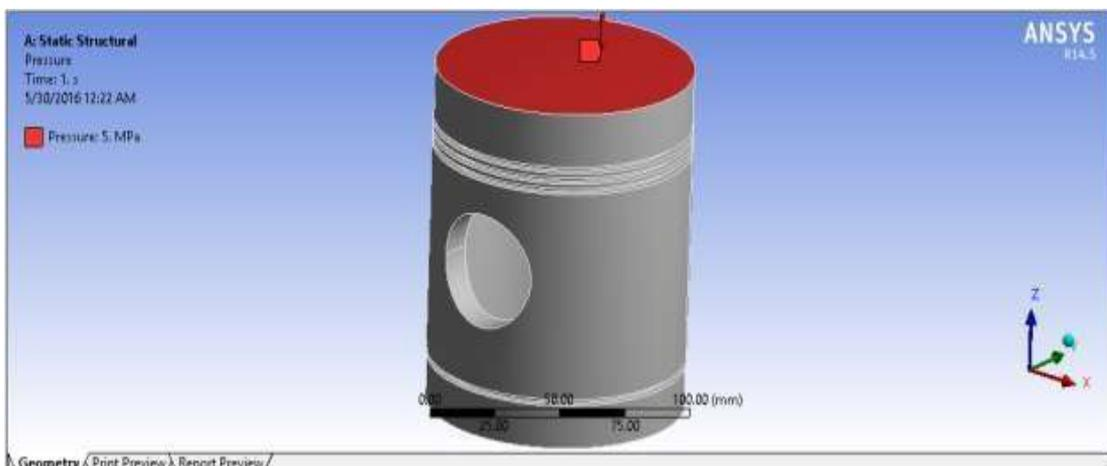
**Fig.5** Applying the pressure on top surface of piston head
