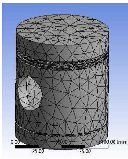
**Fig.3** Meshing of the model in ANSYS 14.5
