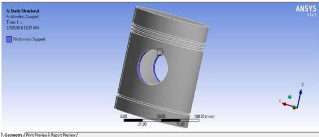
**Fig.4** Restraining the model at piston pin holes
