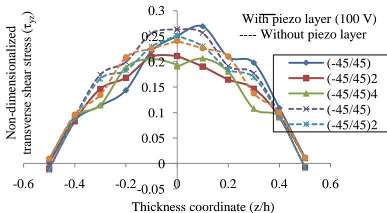
**Fig. 7:** Non-dimensionalized transverse shear stress ( $\tau_{yz}$ ) thickness coordinate ( $z/h$ ) of simply supported anti-symmetric angle-ply piezolaminated plate for model-2
