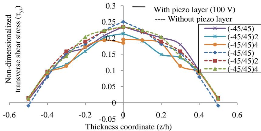
**Fig. 6:** Non-dimensionalized transverse shear stress ( $\tau_{yz}$ ) vs thickness coordinate ( $z/h$ ) of simply supported anti-symmetric angle-ply piezolaminated plate for model-1
