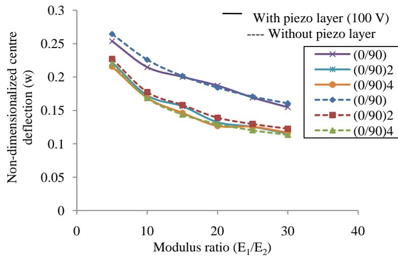
Fig. 3: Non-dimensionalized central deflection ( $w$ ) vs modulus ratio ( $E_1/E_2$ ) of simply supported anti-symmetric cross-ply piezolaminated plate for model-2
