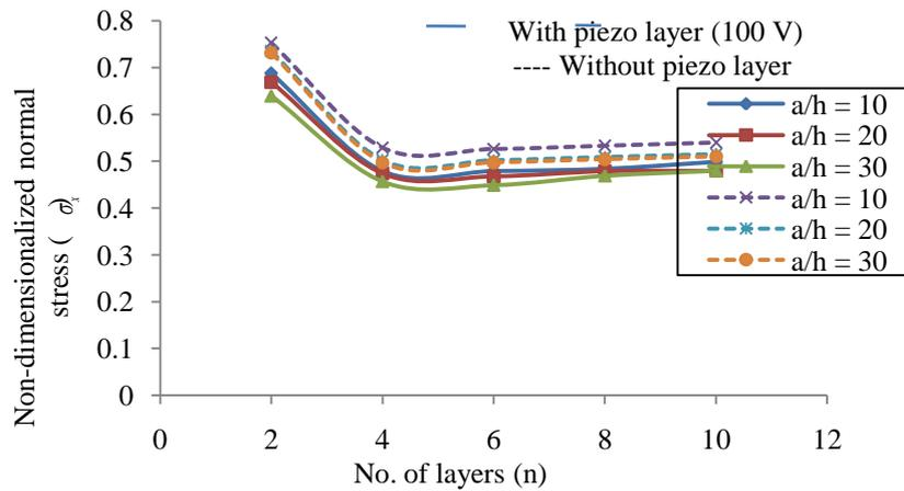
**Fig. 5:** Non-dimensionalized normal stress ( $\sigma_x$ ) vs no. of layers ( $n$ ) of simply supported anti-symmetric cross-ply piezolaminated plate for model-2
