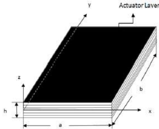
**Fig. 1.** Composite laminated plate attached with piezoelectric layer [5]
