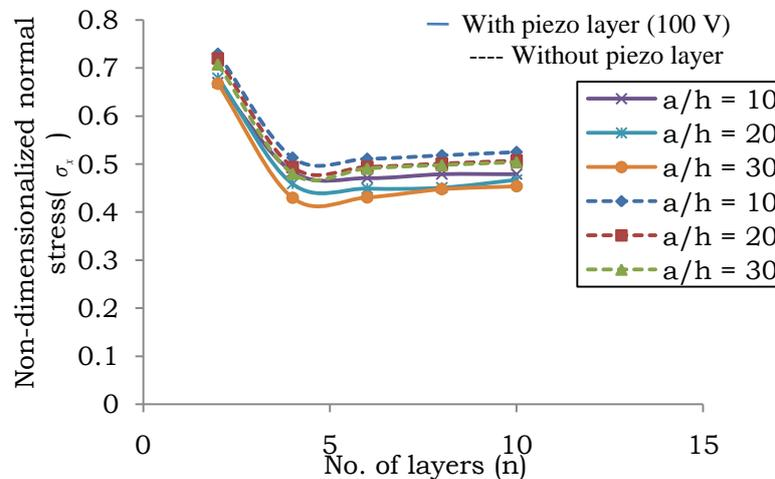
Fig. 4: Non-dimensionalized normal stress ( $\sigma_x$ ) vs no. of layers ( $n$ ) of simply supported anti-symmetric cross-ply piezolaminated plate for model-1
