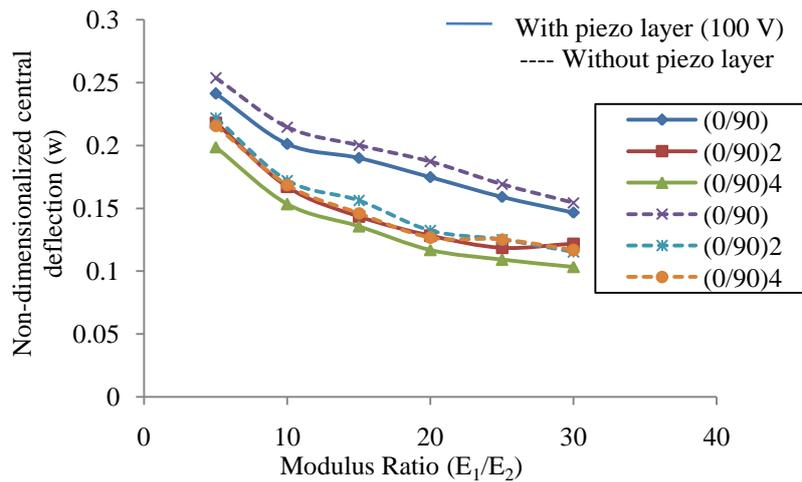
Fig. 2: Non-dimensionalized central deflection ( $w$ ) vs modulus ratio ( $E_1/E_2$ ) for simply supported anti-symmetric cross-ply piezolaminated plate for model-1
