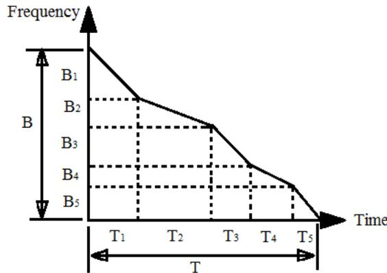
Fig.6. Instantaneous frequency for 5-Stages-LFM waveform
