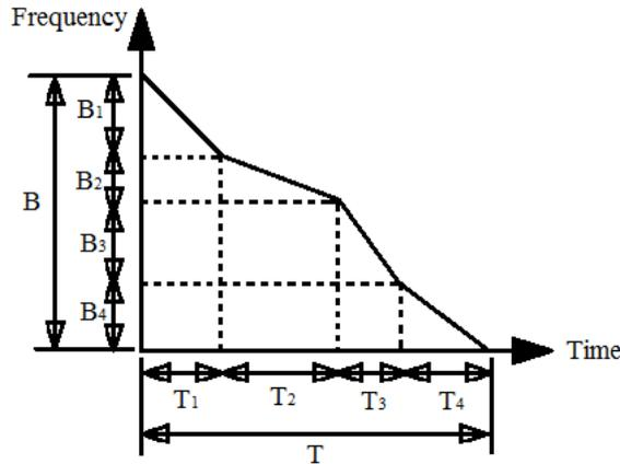
Fig.5. Instantaneous frequency for 4-Stages-LFM waveform
