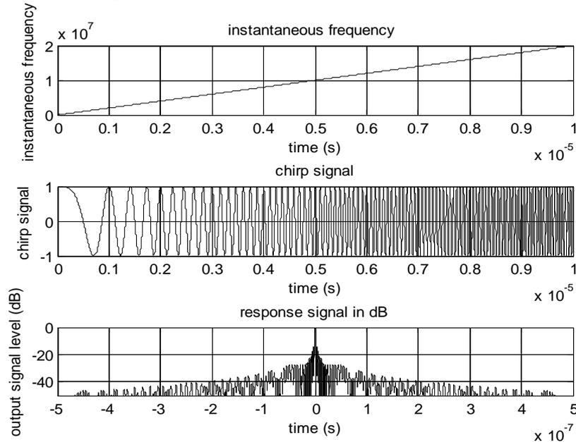
Fig.1. Linear FM waveform.
