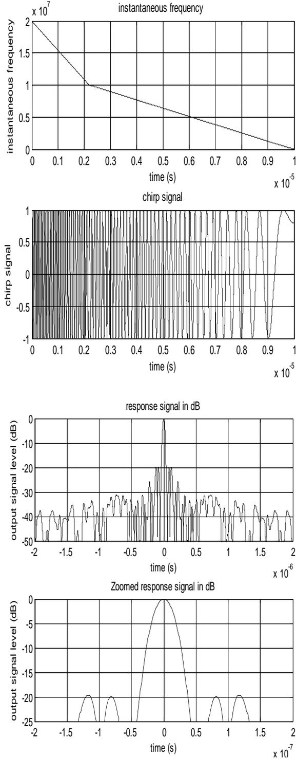
**Fig.7. Modulation signal for Two Stages-LFM waveform with a sidelobe level of -19.65 dB.**
