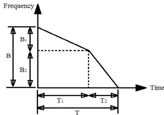
Fig.3. Instantaneous frequency for Two Stages-LFM waveform
