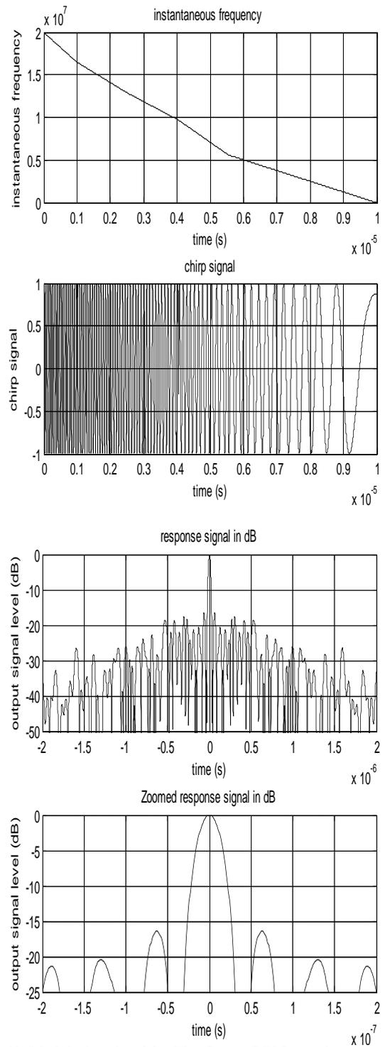
**Fig.10. Modulation signal for Five Stages-LFM waveform with a sidelobe level of -16.4dB.**
