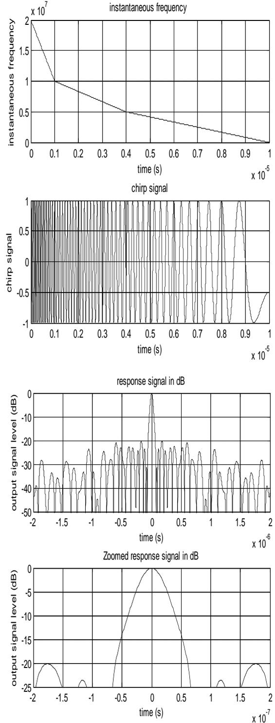
**Fig.8. Modulation signal for Three Stages-LFM waveform with a sidelobe level of -20.15dB.**
