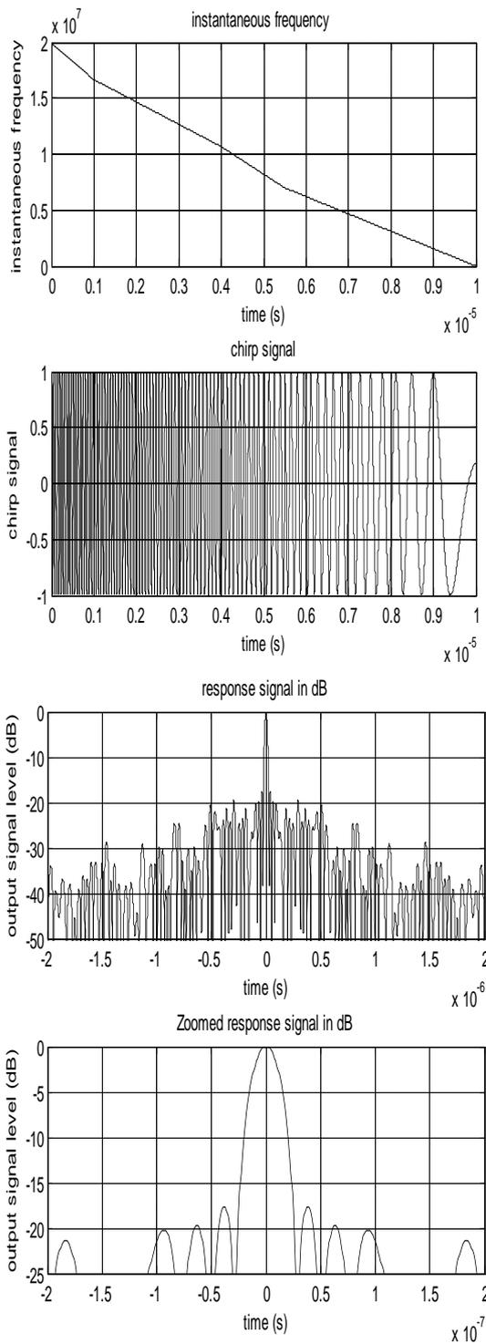
**Fig.9. Modulation signal for Four Stages-LFM waveform with a sidelobe level of -17.6dB.**
