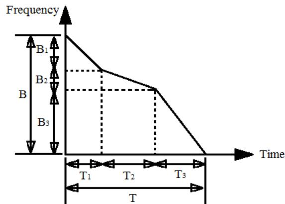
Fig.4. Instantaneous frequency for 3-Stages-LFM waveform
