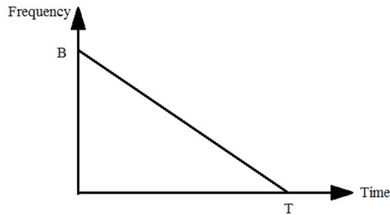
Fig.2. Instantaneous frequency for LFM waveform
