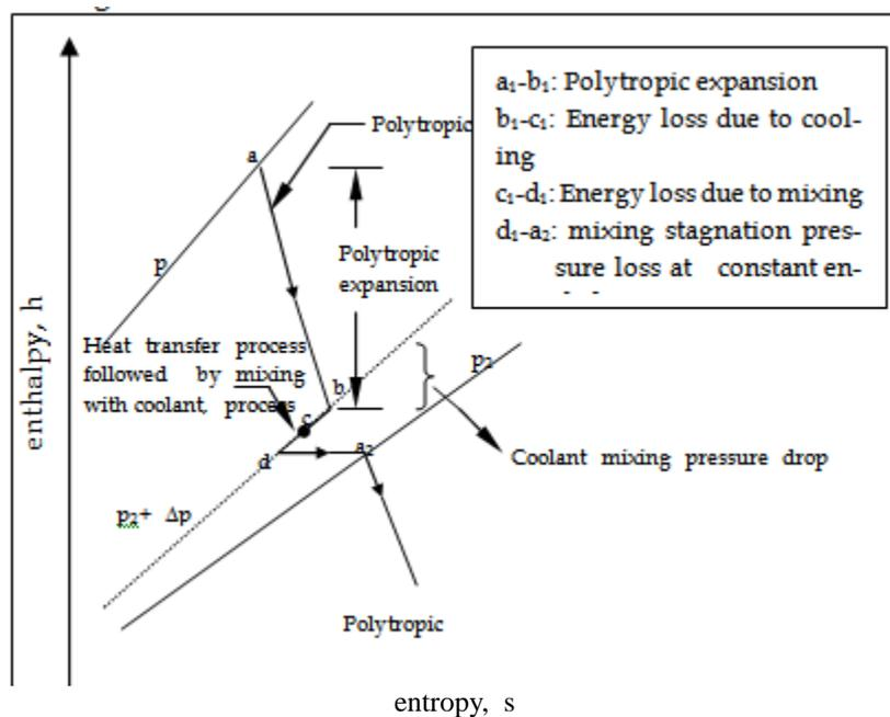
Fig. 2. Expansion path in cooled gas turbine row
