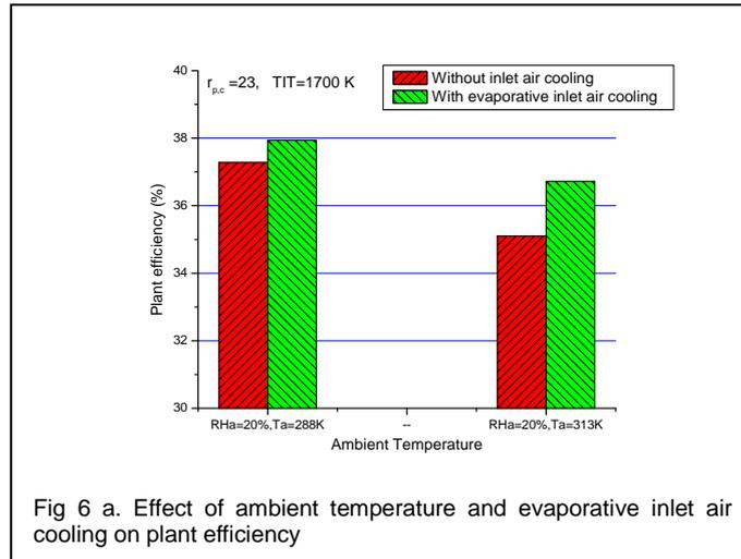
Fig 6 a. Effect of ambient temperature and evaporative inlet air cooling on plant efficiency
