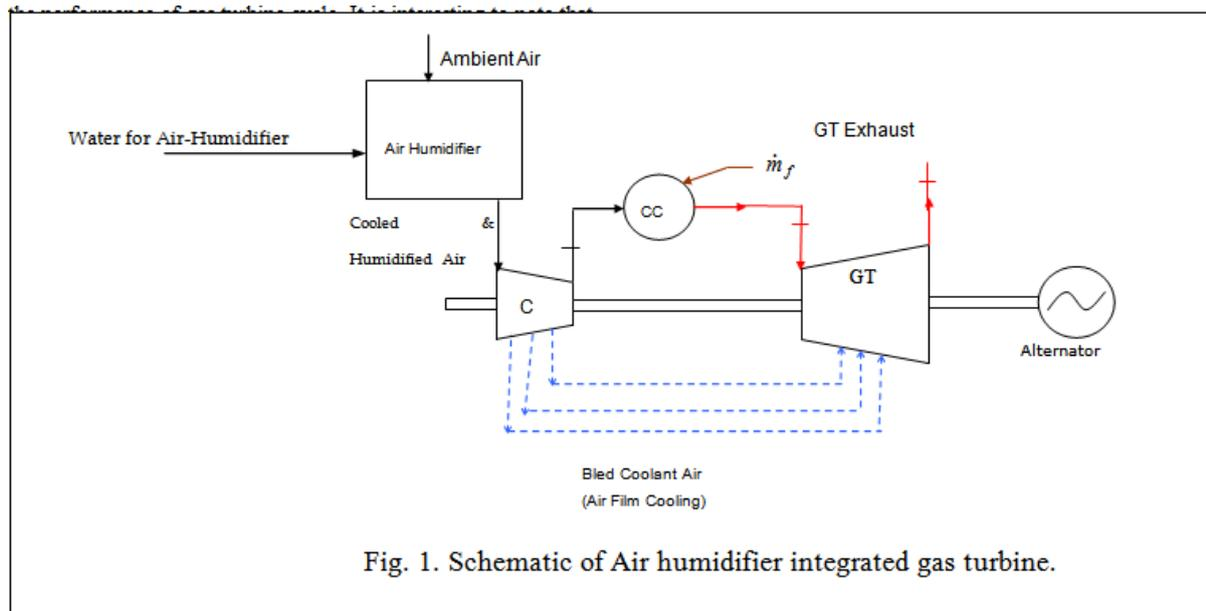
**Fig. 1. Schematic of Air humidifier integrated gas turbine.**
