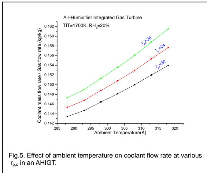
Fig.5. Effect of ambient temperature on coolant flow rate at various  $r_{p,c}$  in an AHIGT.
