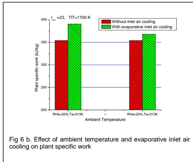
Fig 6 b. Effect of ambient temperature and evaporative inlet air cooling on plant specific work
