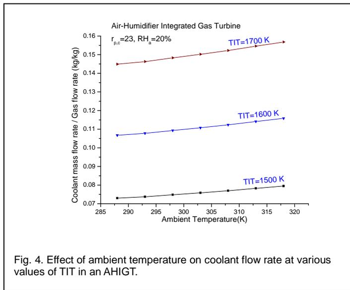
Fig. 4. Effect of ambient temperature on coolant flow rate at various values of TIT in an AHIGT.
