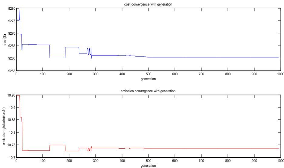
**Figure 2:** Convergence of fuel cost (\$) and gas emissions (ton/h) objective functions (1000MW).
