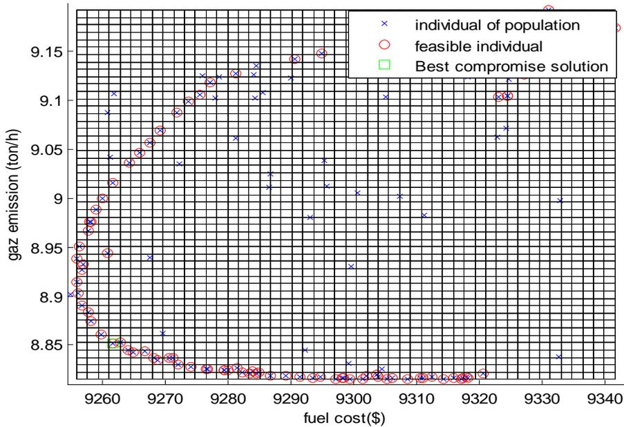
**Figure 5:** Pareto front with the original parameters.
