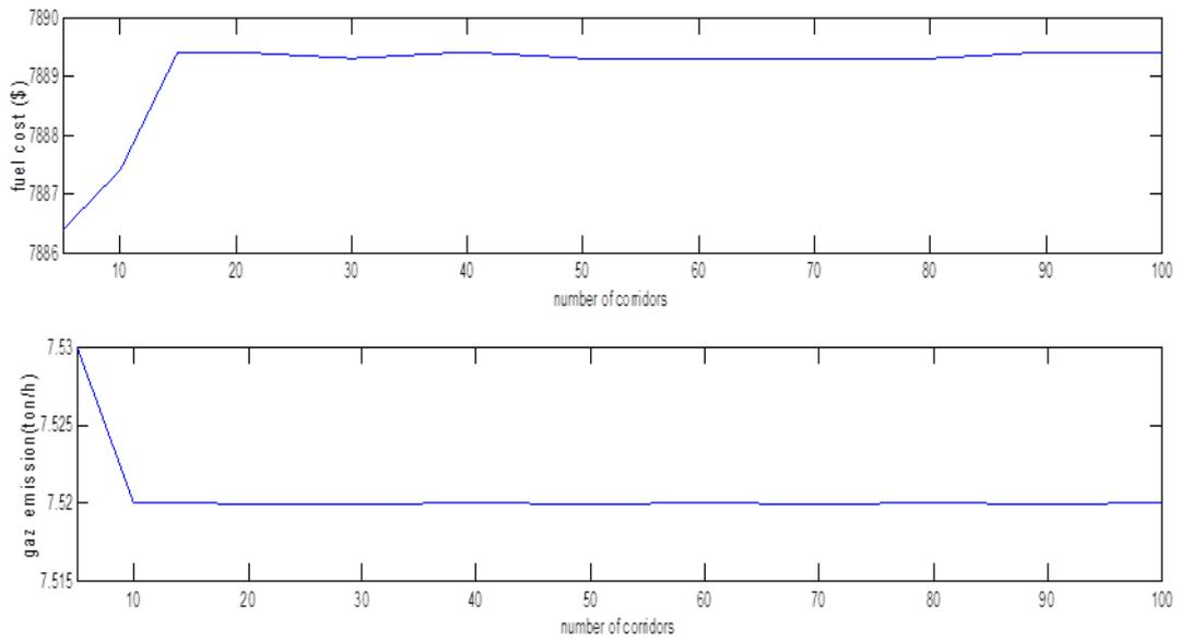
**Figure 3:** Evolution of fuel cost (\$) and gas emissions (ton/h) according to the number of corridors (850 MW). These curves shows that from 20 corridors fuel cost and gas emission are almost uniform. The Pareto front at this value of number of corridors is represented in figure 4.
