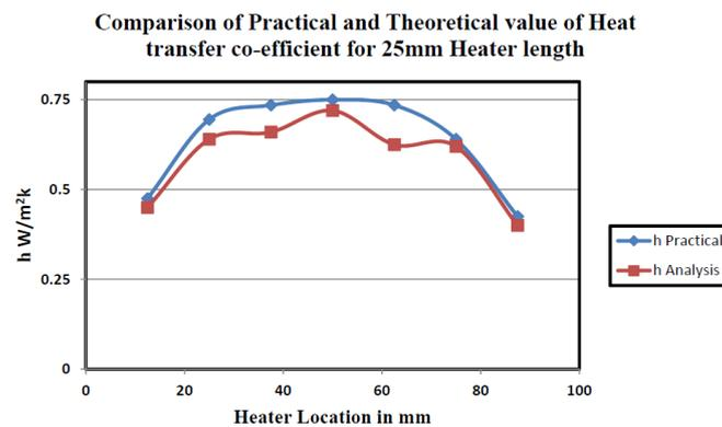
From the graph it reveals that when heater is located lower half of the inner wall heat transfer rate goes on increases and attains maximum value at its mid height, after that it decreases following a symmetry profile at its mid height. The nature of graph remains same for other heater length and locations.
