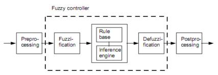
Figure 4: Fuzzy controller structure
