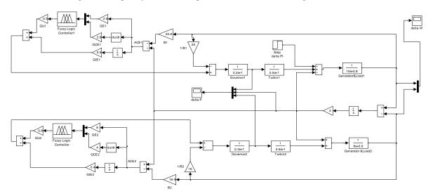
Figure 7: Simulink model of multi- machine power system using FPD+I controller.
