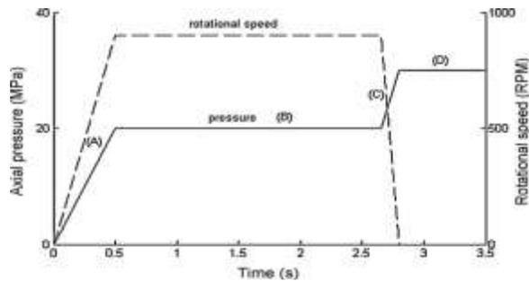
**Fig. 2.** Axial pressure and rotational velocity used in the experiment.
