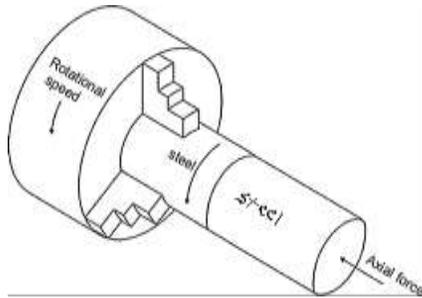
**Fig. 1** Scheme of continuous drive friction welding
