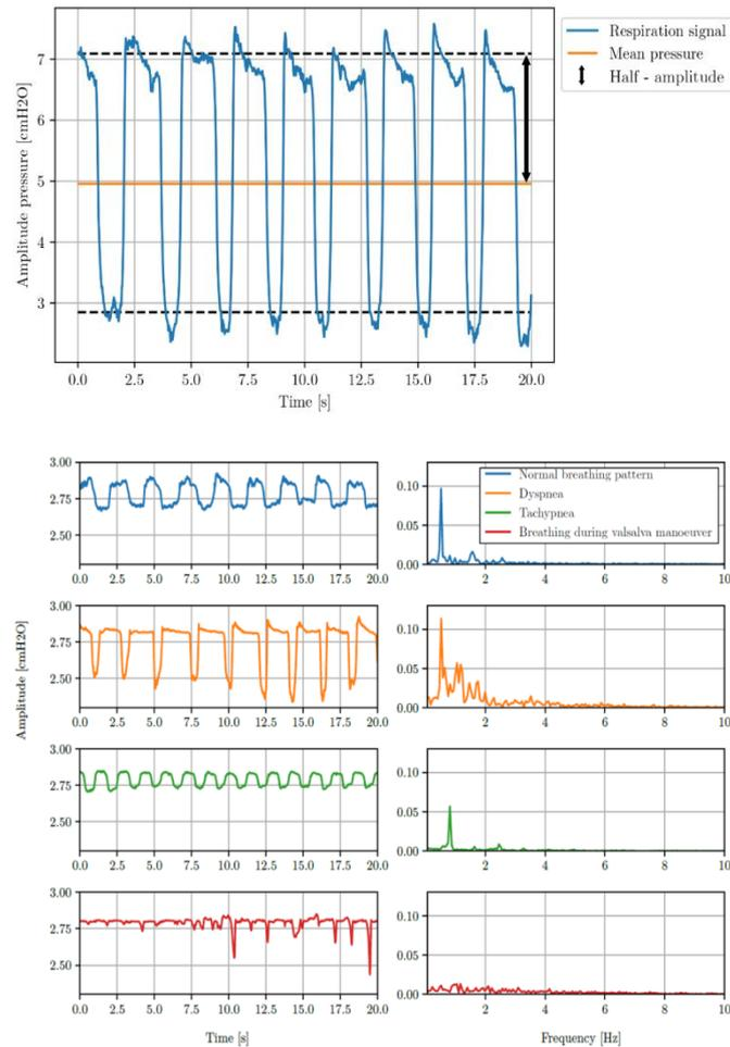
**Figure 2 – (a)** Mean and half-amplitude pressure definition considering a standard respiration signal **(b)** Simulated respirations signals time histories and spectra; Each coloured time-frequency combination stands for each tested simulated respiration
