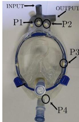
**Figure 3** - Tested masks with installed pressure ports (P1-P4) in the original configuration (ORC) and in the modified configuration (MOC). This is the figure 3 legend: **a)** M1 mask; **b)** M2 mask; **c)** M3 mask **d)** M4 helmet; **f)** M1 mask; **e)** M3 mask; INPUT: 99 entrance O2/air OUTPUT: air outlet where to attach PEEP
