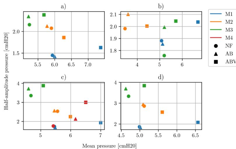
**Figure 6** - Mean values and half-amplitudes of pressure measurements considering M1, M2, M3 masks and M4 helmet, in three different output-conditions at PEEP 5 cmH<sub>2</sub>O (NF = No-filter, AB = Antibacterial filter, ABV = Antibacterial and antiviral filter): **a)** Pressure port P1; **b)** Pressure port P2; **c)** Pressure port P3; **d)** Pressure port P4
