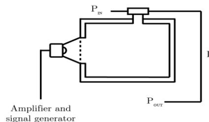
**Figure 1** - Dynamic characterization setup (Pin: Input pressure; Pout: Output pressure; L: Tube length)
