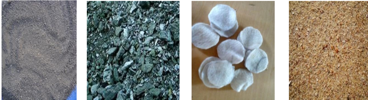
Figure 1(a).Marine clay Figure 1(b).Silica-Manganese slag Figure 1(c). Geo-textile circular discs Figure 1(d). Sand
