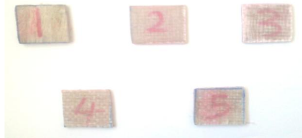
Water absorption test specimen
