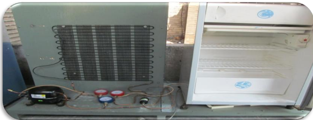
Figure.1 Fabrication of Refrigeration Tutor before Heat Exchanger Incorporation
