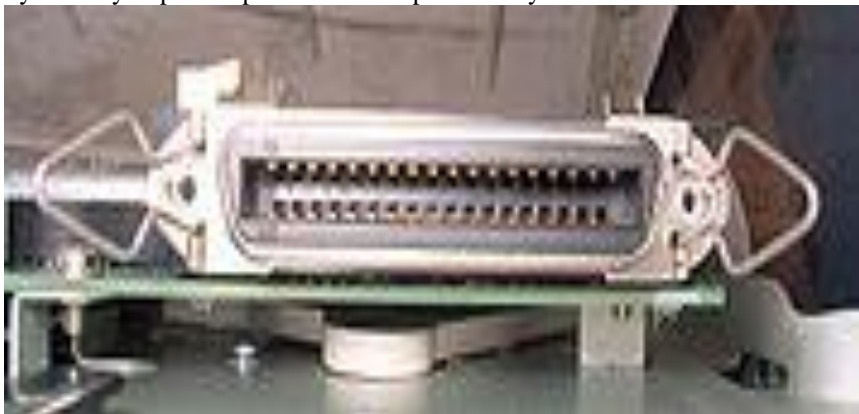
Fig 4 Photo OF A LTP Db25 Printer Parallel Port Head Device
