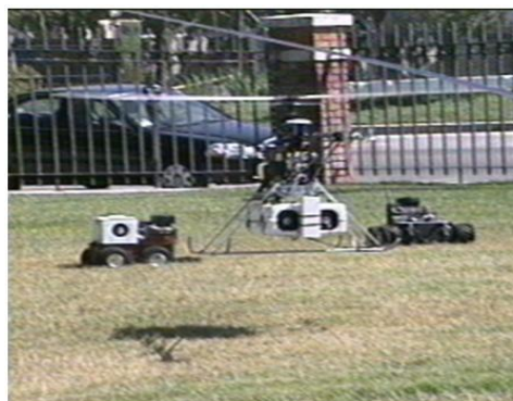
Figure 1: The experimental testbed consisting of the AVATAI (Autonomous Vehicle Aerial Tracking and Inspection) robot helicopter and two Pioneer AT mobile robots.
