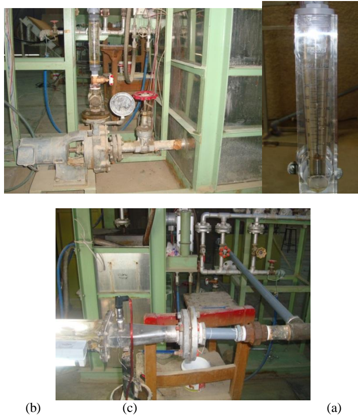
Figure 2. (a) Water system, (b) Air flow meter, (c) Enlargement connecting part, flange, piping system and pressure transducer sensor [13]-[14].
