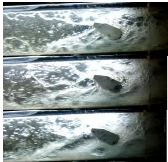
(b) Figure 10. Photographs for the two phase flow behavior at Q_w=45 l/min, angle of attack= 0 degree and Q_a=10, 20, 30, 40 l/min respectively.
