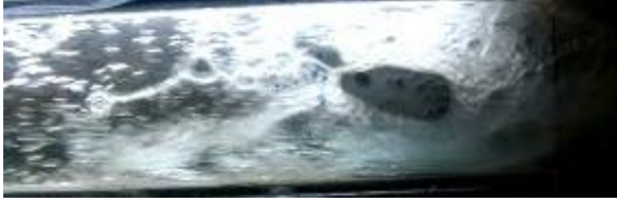
(c) Figure 11. Photographs for the two phase flow behavior at Q_w=45 l/min, angle of attack= 15 degree and Q_a=10, 20, 30, 40 l/min respectively.
