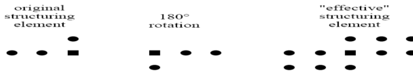
Figure 3. Illustration of an “effective” structuring element of opening and closing formed by rotation between successive erosions and dilations. Squares (■) denote the origin of the plane; circles (●) denote other points in the set. The opening and closing operations are also complementary, and when applied in sequence, they form the doubly compound morphological operators open-close (OC) and close-open (CO):
