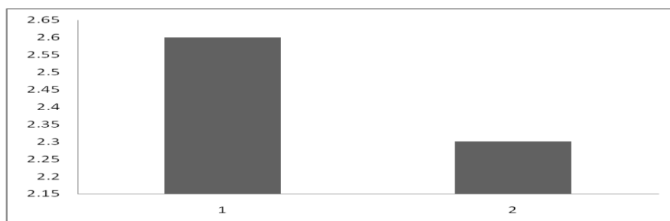
Figure 1 Tensile strenght of peroxide cured pure EPDM before and after thermal ageing; 1. unaged and 2. Aged
