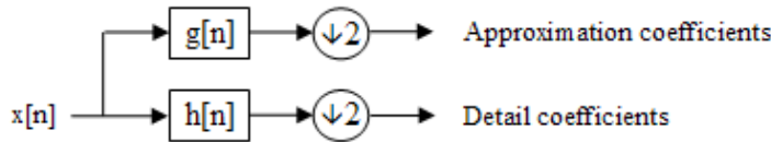
Figure 6: Block diagram of filter analysis
