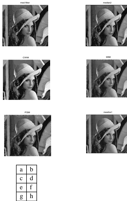
Fig 1 . (a) Original image (b) Noisy image with noise density of 20% (c) Output of Median I (d) Output of Median II (e) Output of CWM (f) Output of MSM (g) Output of PSM (h) Fused Output
