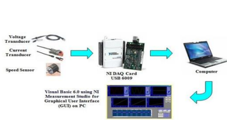
Fig 1.2: Monitoring of motor using DAQ Motor Monitoring
