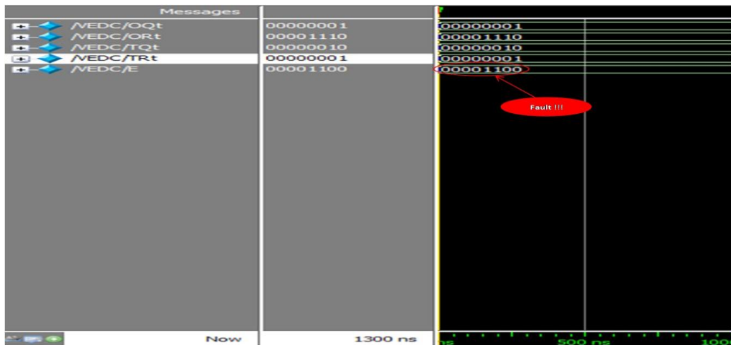
Figure 6. Simulation Result of Fault Detection Circuit identifying the fault using RP Codes and Test Codes for a Specific PE in a Motion Analysis Process
