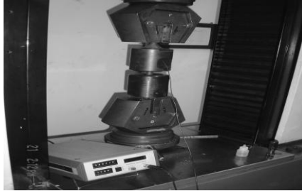
Figure 8: Bolt Calibration setup
