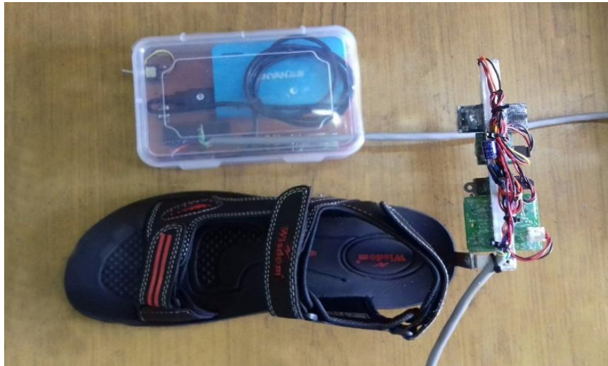
Fig.1. Footwear consisting of five sensors at the backside
