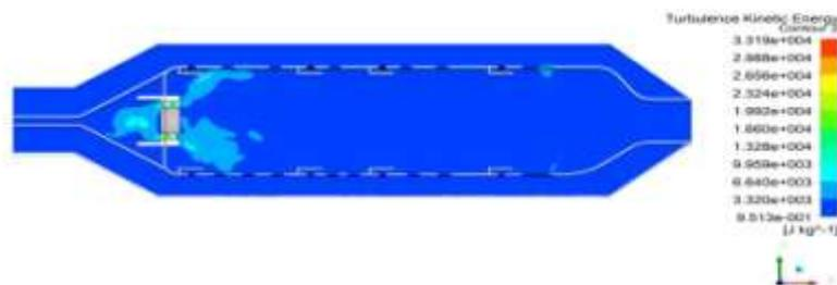
Fig 12.0 Contour of turbulent kinetic energy, case 1
