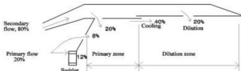
Fig 4.0 Apportioning of combustion air
