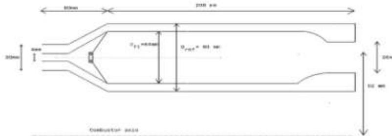
Fig 1.0 Schematics of basic combustion chamber
