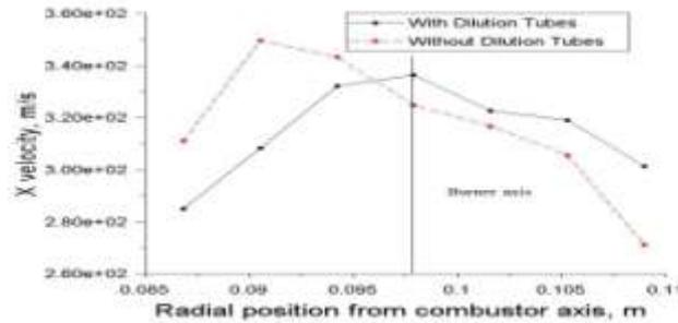
**Fig 6.0** X velocity component
