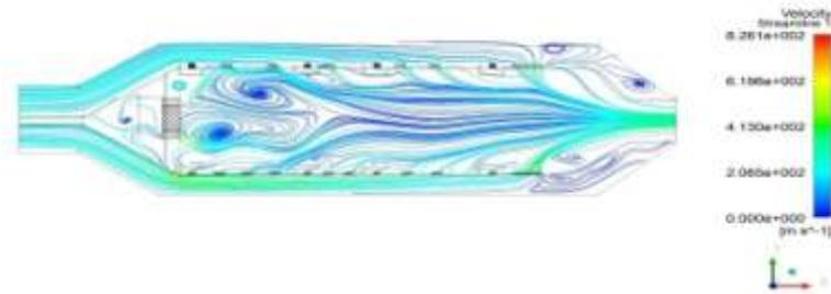
Fig 9.0 Streamlines in combustor, Case 1
