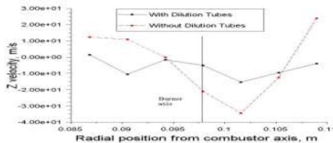
**Fig 8.0** Z velocity component
