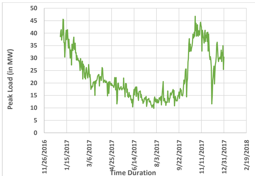
Figure 1 Load Curve Graph for 132 KV Substation
