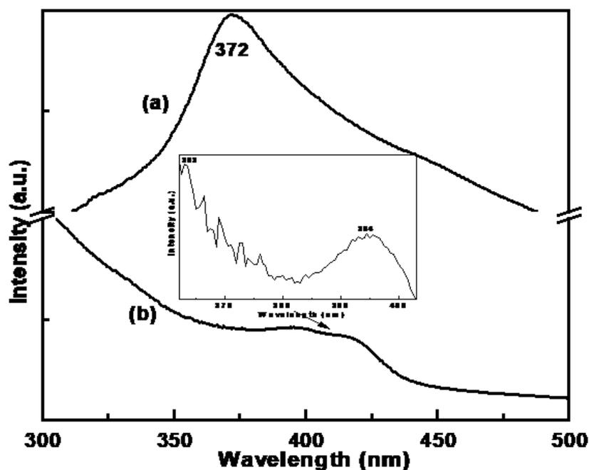
Figure 5: PL spectra of Cobalt doped ZnO sample.
