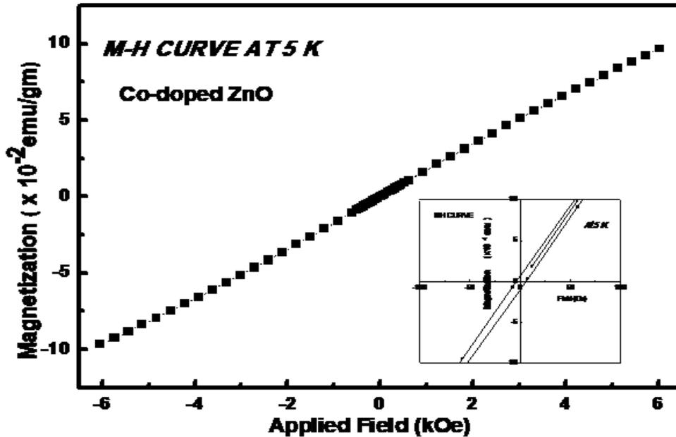
Figure 3: Magnetization versus applied field (M-H) curve at 5 K of Cobalt doped ZnO sample.
