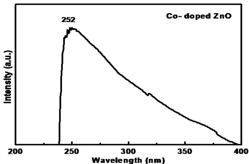
**Figure 2: UV-Visible absorbance spectra of 5 % Cobalt doped ZnO sample.**
