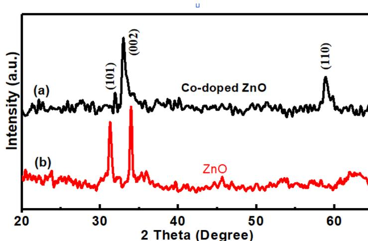
**Figure 1: XRD spectra of samples; (a) Un-doped and (b) Cobalt doped ZnO.**
