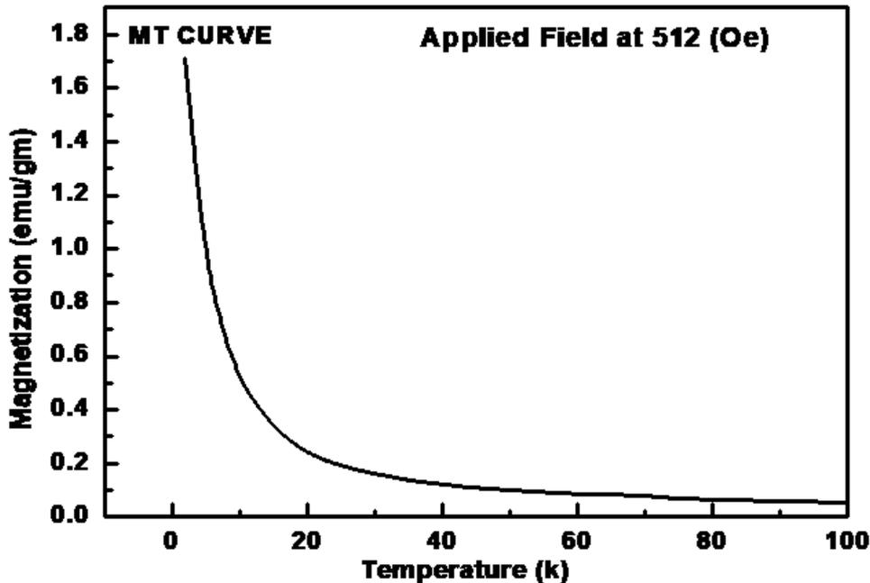
Figure 4: Temperature dependent magnetization (M-T) curve at 512 (Oe) of Co-doped ZnO Sample.
