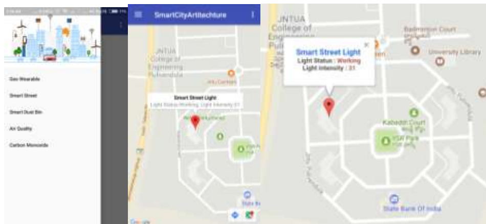
Figure 5. Smart street light, working status and intensity at daytime in mobile application and web application
