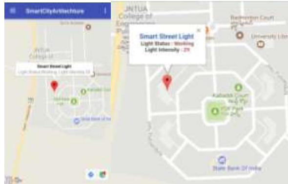
Figure 6. Smart street light, working status and intensity at night time in mobile application and web application
