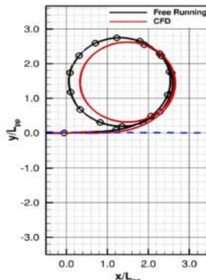
Fig 16: Turning circle simulation and validation with free running test
