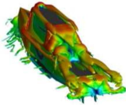
Fig11: Simulation of wind effect over superstructure
