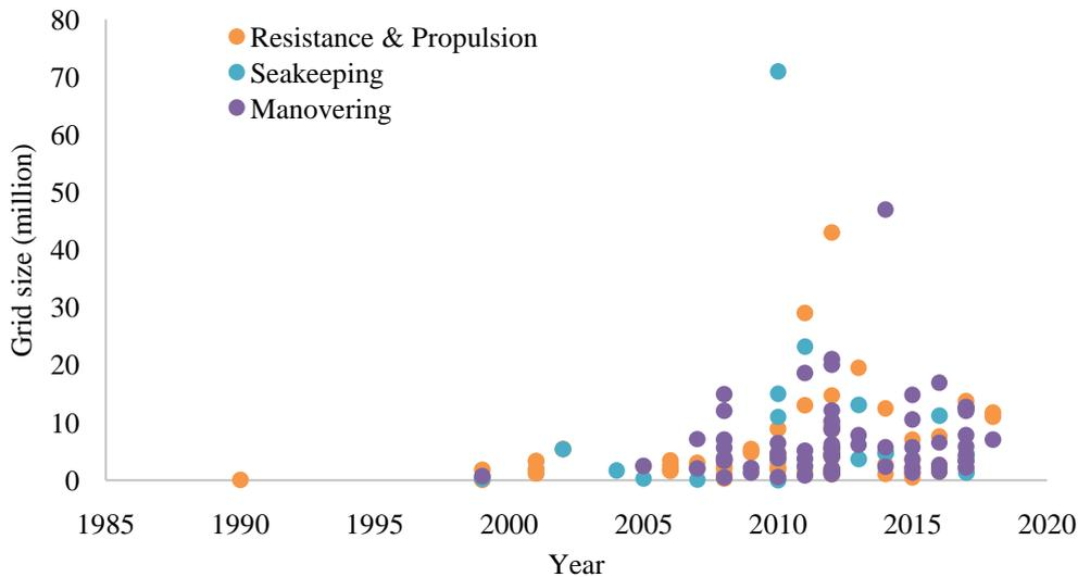
Fig 6: Evolution of grid size for ship hydrodynamic CFD simulations
