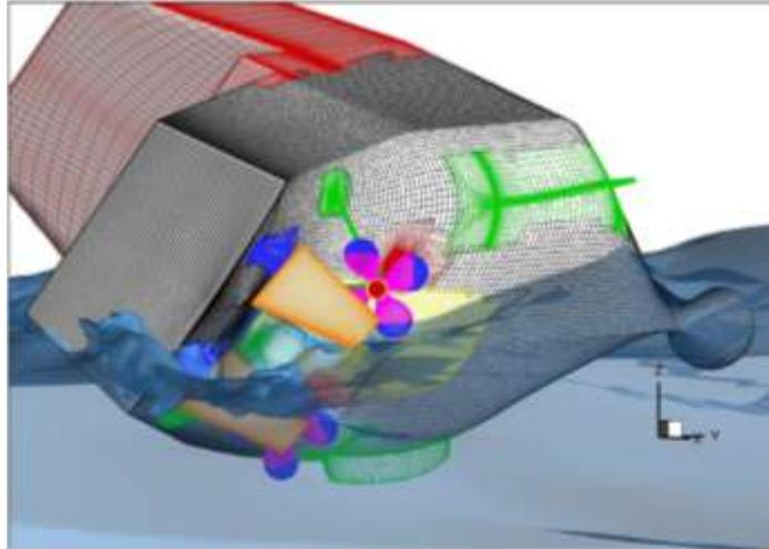
**Fig 8:** Application of overset strategy for rotating propeller and moving rudder [65]
