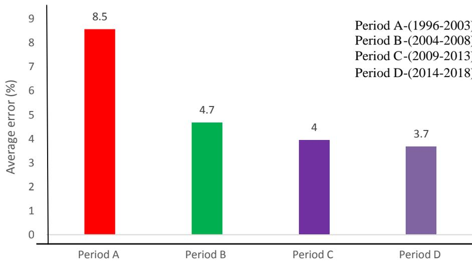
Fig 13: Average error comparison for resistance and propulsion using CFD method
