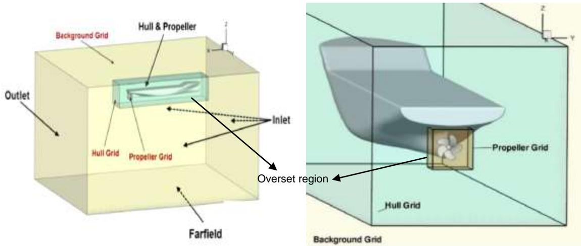
Fig 4: Dynamic meshing strategy applied for ship propulsion[20]
