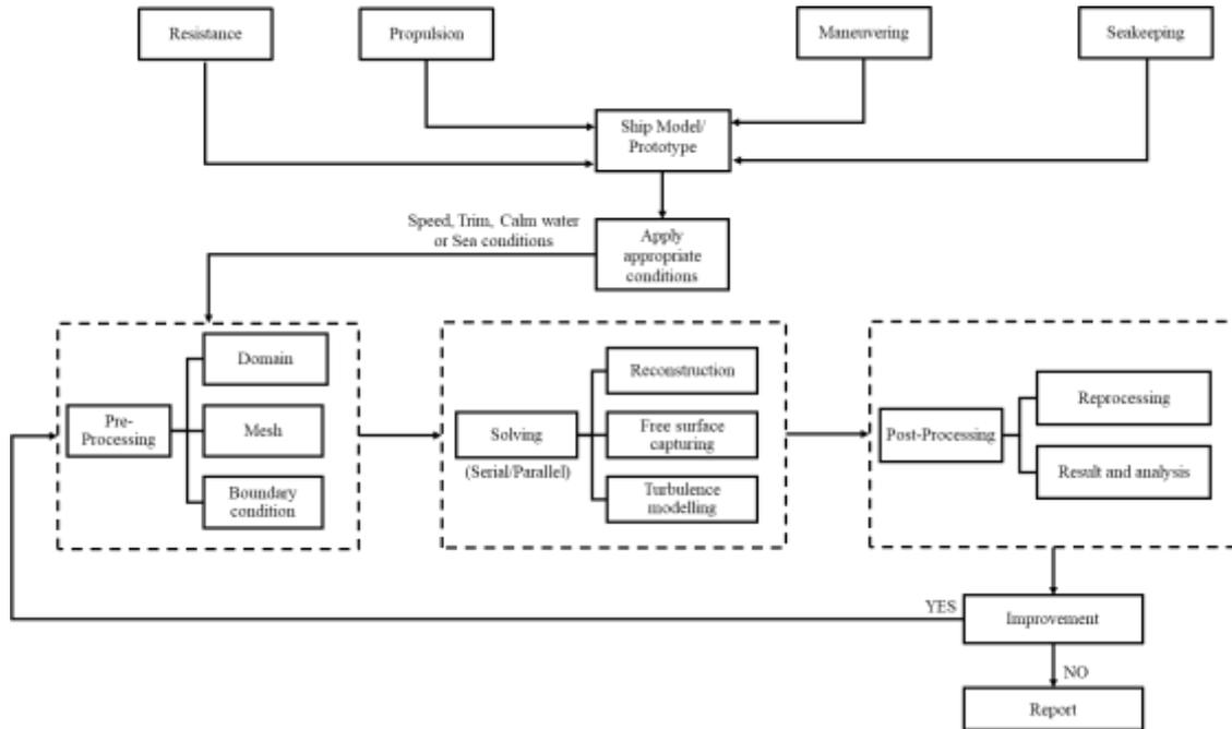
Fig 3: CFD procedure to obtain a typical ship hydrodynamic solution
