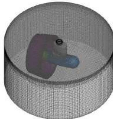
**Fig 10:** Cylindrical sub domain around the propeller for dynamics
