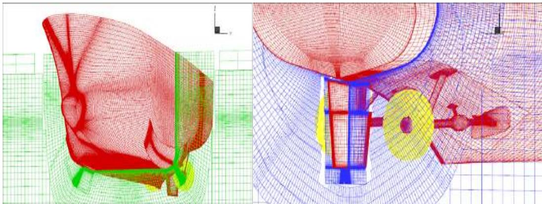
Fig 5: Generation of overset grid for turning circle simulations
