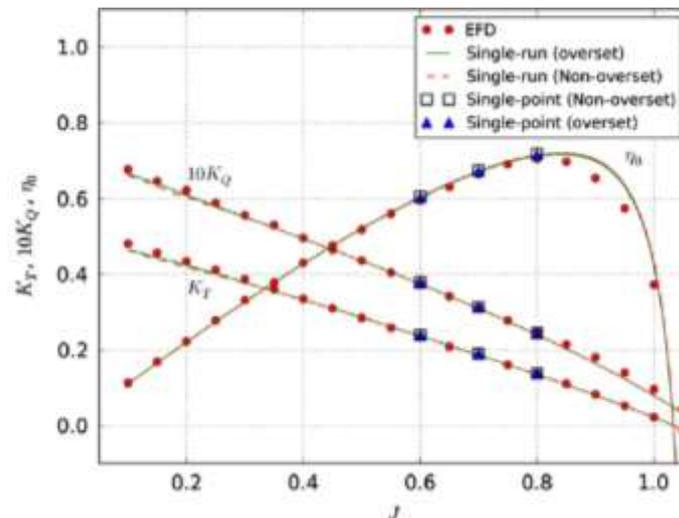
Fig 7: Comparison of overset with non-overset grid approach [15]
