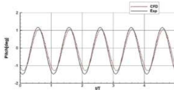
Fig 15: Typical result for pitch motion
