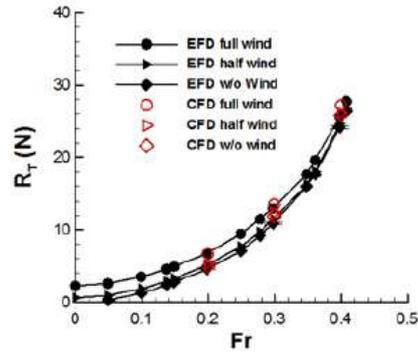
Fig 12: Comparison of CFD with EFD for total resistance
