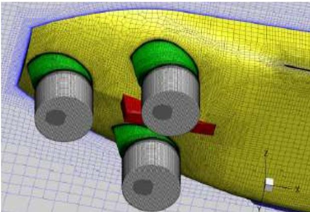
**Fig 9:** Mesh around the aft of drill ship for 3 azimuthing propeller
