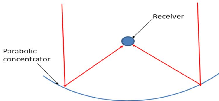
Fig. 1 Schematic of the parabolic trough collector
