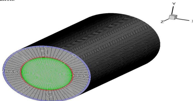
**Fig. 4** Mesh of PTC receiver
