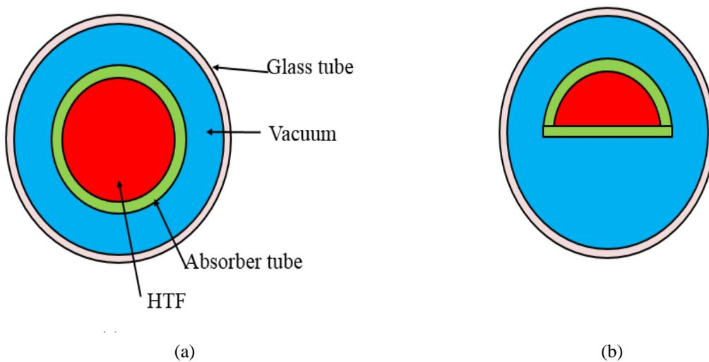
Fig. 2 Cross sectional view of receiver (a) circular absorber tube (b) semicircular absorber tube
