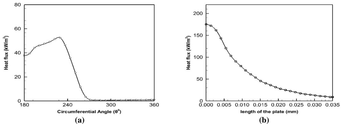
Fig. 5 Distribution of heat flux over absorber tube (a) Circular (b) Semicircular
