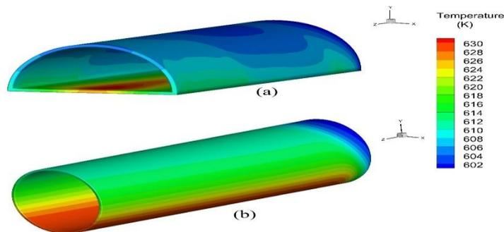
Fig. 6 Temperature distribution over (a) semicircular absorber tube (b) circular absorber tube
