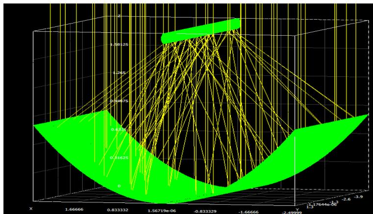
**Fig. 3** Sample ray tracing in SolTrace
