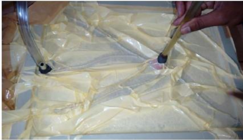
Figure 1. Resin transfer in VARTM.
