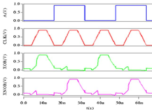
Fig. 7. Transient response of the proposed adiabatic hybrid MTJ/CMOS full adder circuit. Here it is assumed that the input “ B” is logic “ 1” and stored in MTJs.
