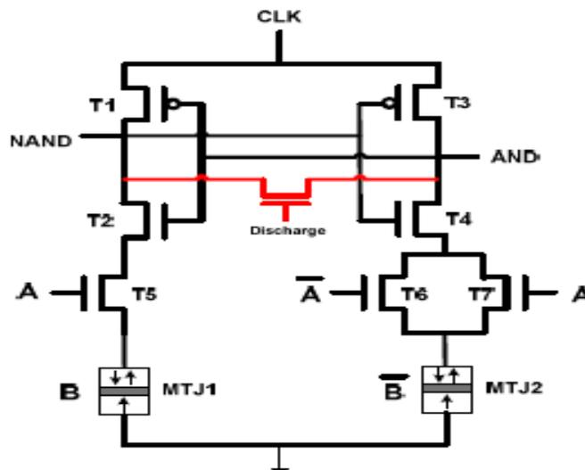
Fig.4 Proposed adiabatic hybrid MTJ/CMOS AND/NAND.
