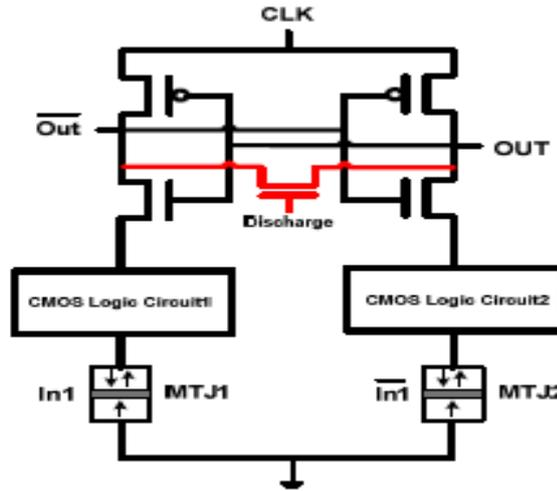
Fig.3: General schematic of the proposed adiabatic hybrid MTJ/CMOS design.
