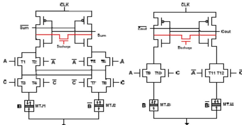
Fig.6: Proposed adiabatic hybrid MTJ/CMOS full adder design.
