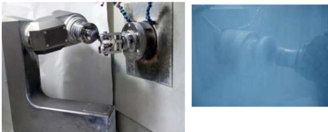
Figure 8. Bonnet polishing. Figure 9. Fluid jet polishing.
