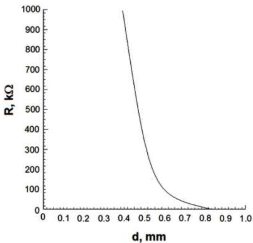
**Figure 11.** The resistance dependence on sample thickness. Treatment is by alternating magnetic field at  $T=85^{\circ}\text{C}$ .
