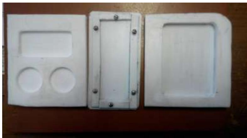
Figure 1. Teflon press-forms for preparation of different size films.
