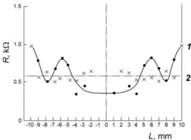
Figure 17. Polymer composite C/Co, wt. 30%; 1: resistant distribution in the sample as a result of treatment; 2: resistant in the sample before the treatment.
