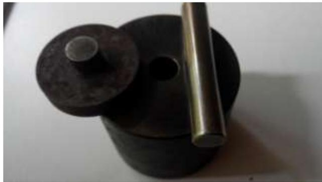
Figure 6. Press form for samples fabrication.
