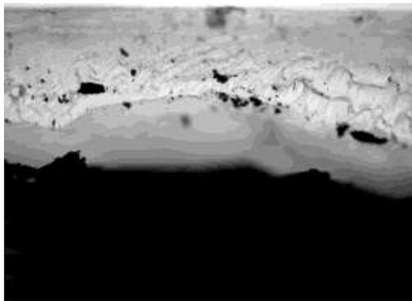
**Figure 14.** Treatment of C/Cwt.50% sample without magnet at  $T=85^\circ\text{C}$  during 2.5 hours.
