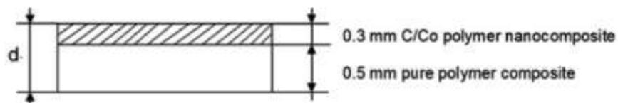
Figure 7. Experimental polymer pile.
