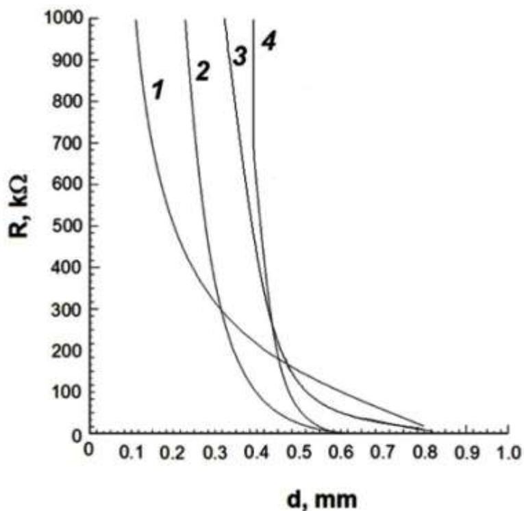
**Figure 12.** The resistance dependence on sample thickness (summary): Curve 1 corresponds to one given in **Figure 8**; Curve 2 corresponds to one given in **Figure 9**; Curve 3 corresponds to one given in **Figure 10**; Curve 4 corresponds to one given in **Figure 11**.
