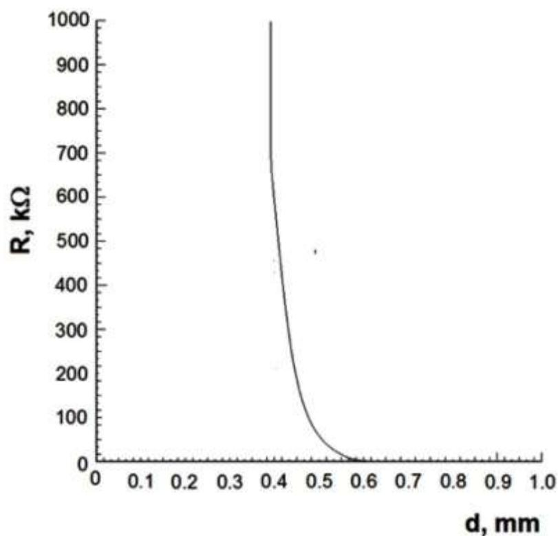
**Figure 10.** The resistance dependence on sample thickness. The treatment is without magnetic field at  $85^{\circ}\text{C}$ .
