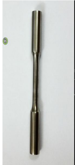
Figure 1: Tensile test specimen with dimension in mm.
