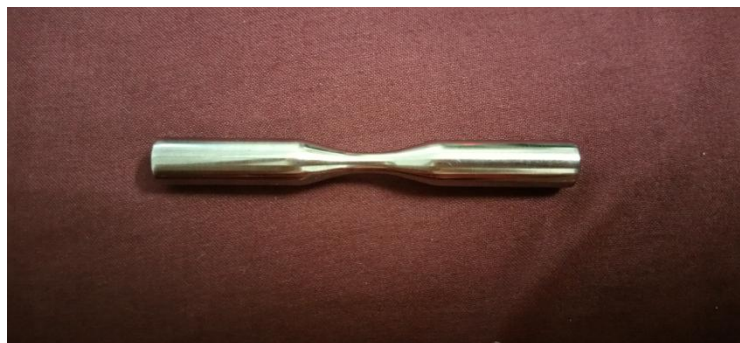
Figure 2: Rotating bending fatigue testing specimen.
