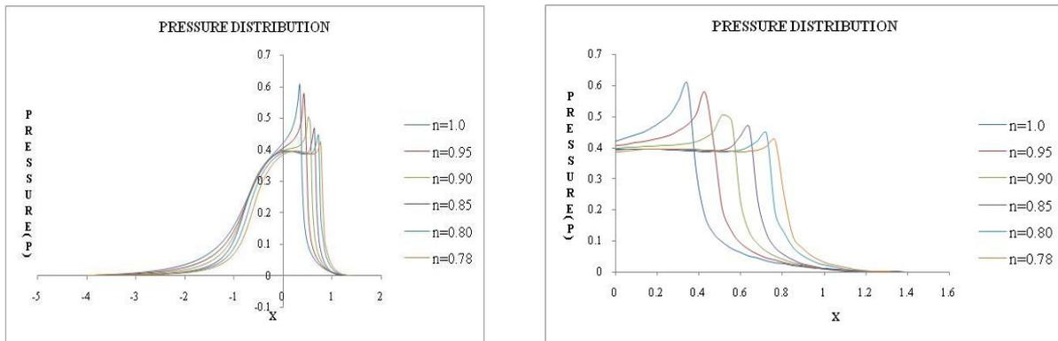
Figure 2(a) Comparison of pressure distribution and spread of pressure spike for fixed low-load ( $W$ ), high-speed ( $U$ ),  $G$  and varying rheological parameter  $n$
