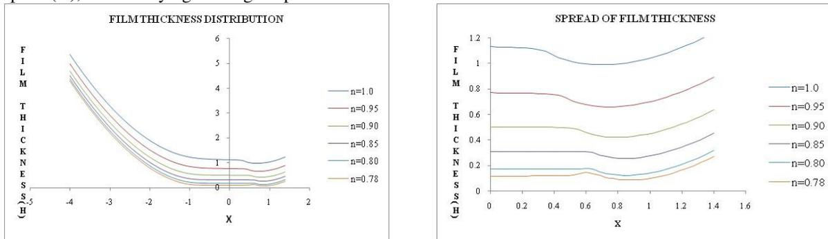
Figure 2(b) Comparison of film profile and its spread for fixed low-load ( $W$ ), high-speed ( $U$ ),  $G$  and varying rheological parameter  $n$
