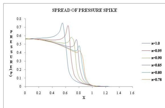
**Figure 1(a)** Comparison of pressure distribution and spread of pressure spike for fixed high-load ( $W$ ), low-speed ( $U$ ),  $G$  and varying rheological parameter  $n$
