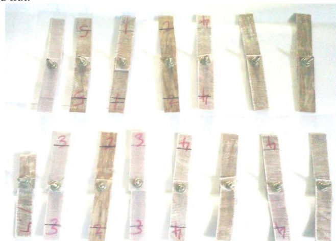
Tensile test specimen with bolt joint
