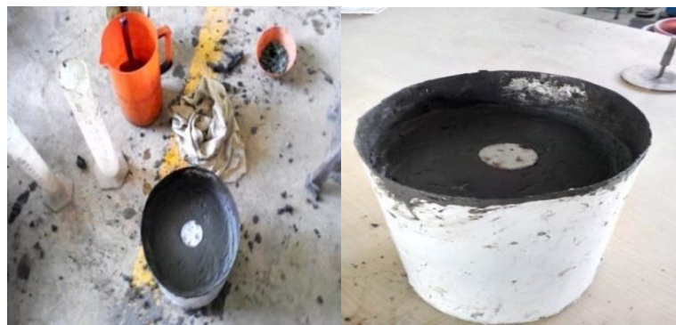
Figure 4. Placing of geo-textile circular discs
