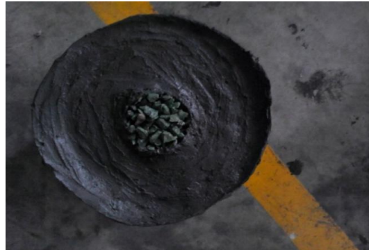
Figure 3. Ordinary floating Stone Column
