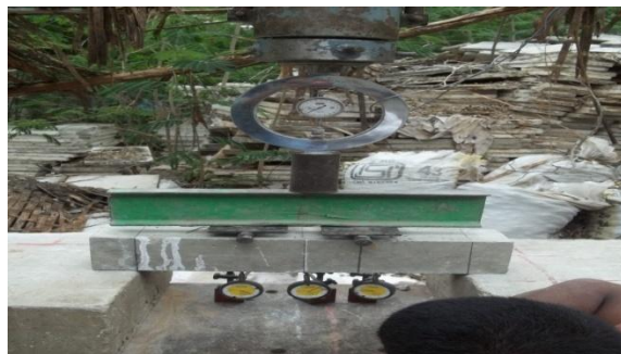
Plate 8: Test Set Up For Flexural Strength Before Testing
