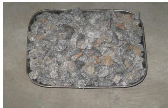
PLATE 7. NATURAL COARSE AGGREGATE
