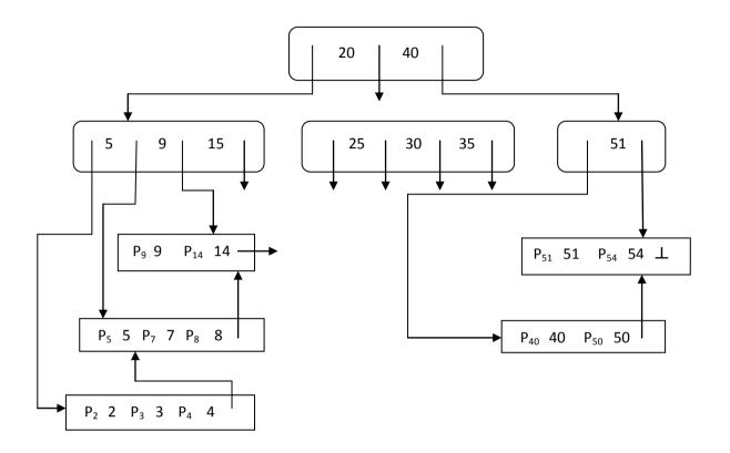
Example2: In the B<sup>+</sup>-tree of example1, let us insert an entry for Books 1. The original contents of the leaf node (with the label  $PT_0$ ) in which the key would be inserted are:
