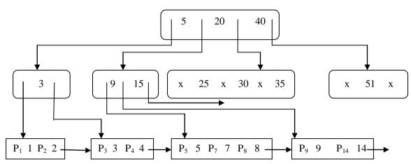
Let the address of the new node be  $P_Y$ . Then the pair < 5,  $P_Y$  > is passed to the parent node for insertion. Figure 2: The B<sup>+</sup>- tree of example1 after insertion of the key for Books1.
