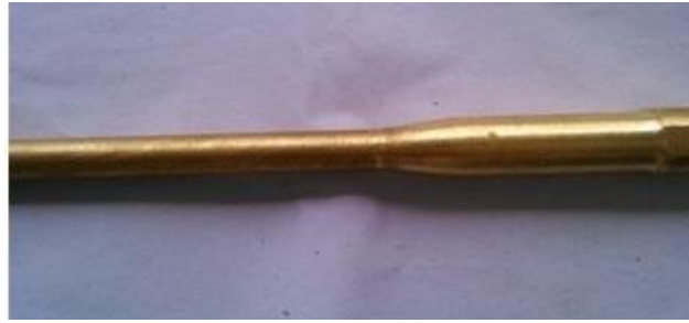
Figure 3.3.4.2-Annealed fatigue test pieces of brass materials
