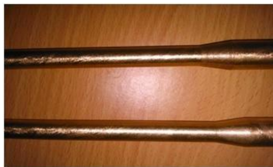
Figure 3.3.6.1 –Corroded fatigue test pieces of brass material
