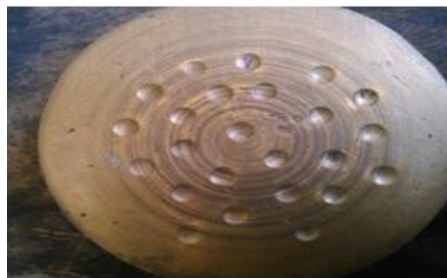
Figure 3.3.3.2 –Brass specimen indentation after Brinell hardness test.
