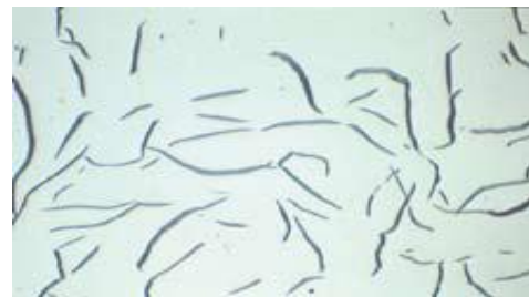
Fig-1 SEM image of grey iron with flake graphite Fig. 2: Well-polished graphite flakes
