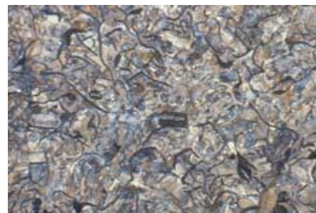
Fig. 3b Grey iron with flake graphite in 200x
