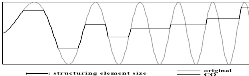
Figure 7. Effect of close-opening (CO) on a 1-D frequency-modulated signal.
