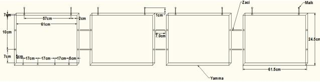
Figure 4. The use of Zaki and Maik in the construction, and how the four Yammas were coupled together
