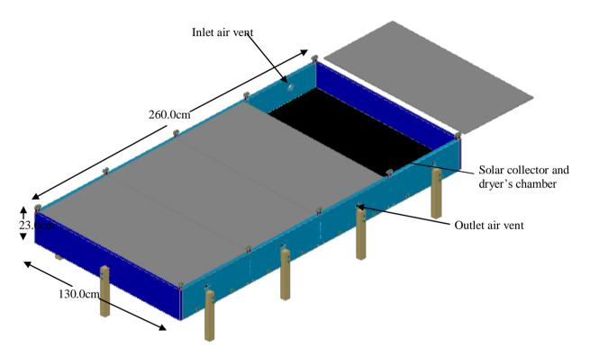
Figure 2. The Pictorial view of Solar Food Dryer. As seen in figure
